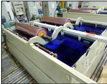
Fig 7 The copper bath, which uses a similar procedure to the nickel and chrome baths.
