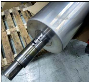
Fig 8 A cylinder after receiving its primer layer of nickel.
