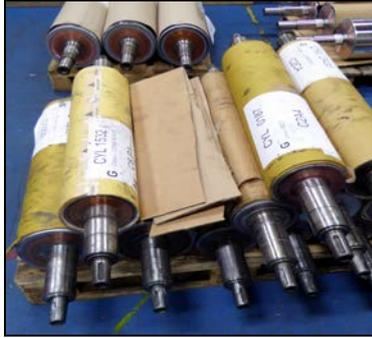
Fig 5 Cylinder deliveries back from the printers, covered with grease and ink and awaiting processing.
