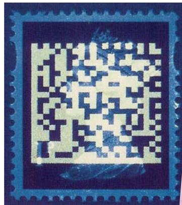
An unadopted example of 3D bar-coding using luminescence, viewed under UV light
