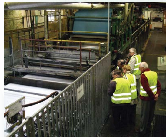
The Fourdrinier paper-making machine at Frogmore Paper Mill in Apsley, Hertfordshire
