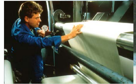
A Harrison employee ensuring that the coated paper surface is smooth prior to rewinding, 1975
