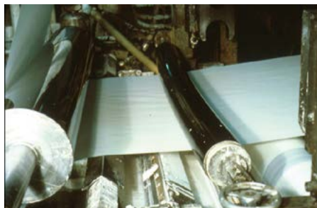
Applying the coating to the base paper, 1975. Note the bow roller keeping the paper in close contact with the coating head
